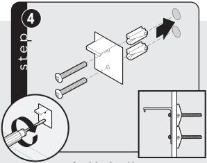
Attach bracket with mounting hardware provided.
